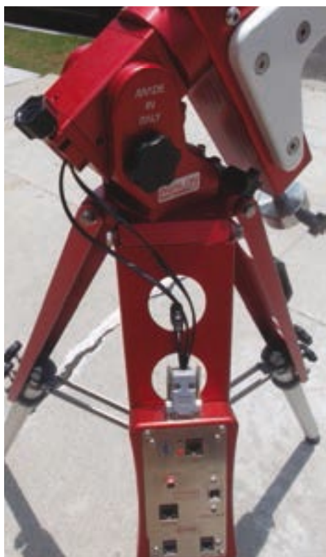
Image 9 - Clean cable management is facilitated by the RA through-bore port.
