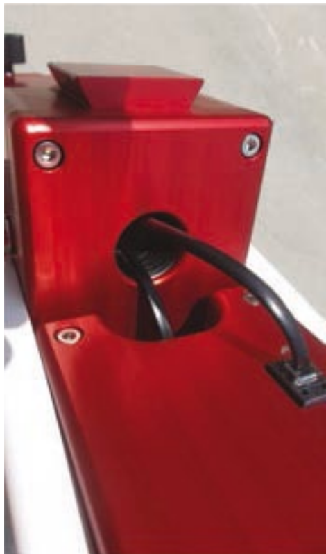
Image 10 - Power and camera cables can also be routed through the RA bore.
