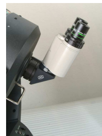
Mark V Großfeld- Binokular am C8 GPS: BTA (#21), T-2 Zenit- prisma (#1b), Mark V (#2456410)
