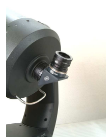
Celestron C8 GPS: BTA (#21), Maxbright-Zenit- spiegel (#1a), T-2 Schnellwechsellvorrichtung (#6&7), ClickLock® (#8)
