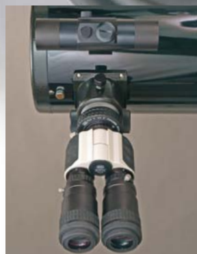
Maxbright-Bino am 8" Newton, – 2" Four-in-One-Adapter, 2" Newton-Komakorrektor 1.7x, 5 mm Hyperion-Okulare, Baader Skysurfer V Visiersucher
