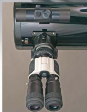
Maxbright-Bino, 8" Celestron-Newton, 5mm Hyperion, Baader Foresight in one Ultrashort-Adapter, 2" Bino Coma Corrector 1.7x, Baader Sky Surfer V Foursight
